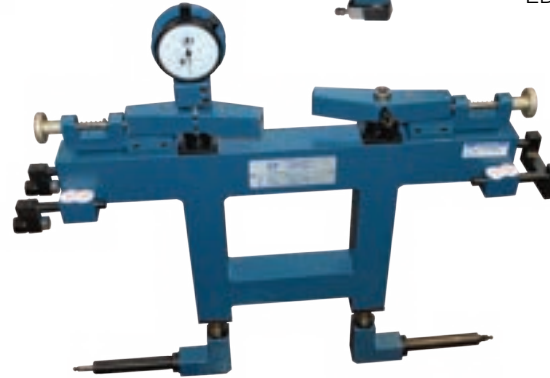
LD - Swing gage, where the heads rotate inward for long retraction
