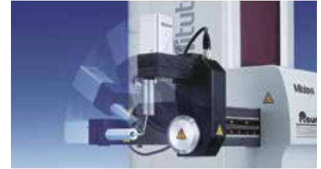
Holder-arm orientation switching (vertical position - horizontal position)
