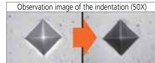
Stray light reduction around the indentation
